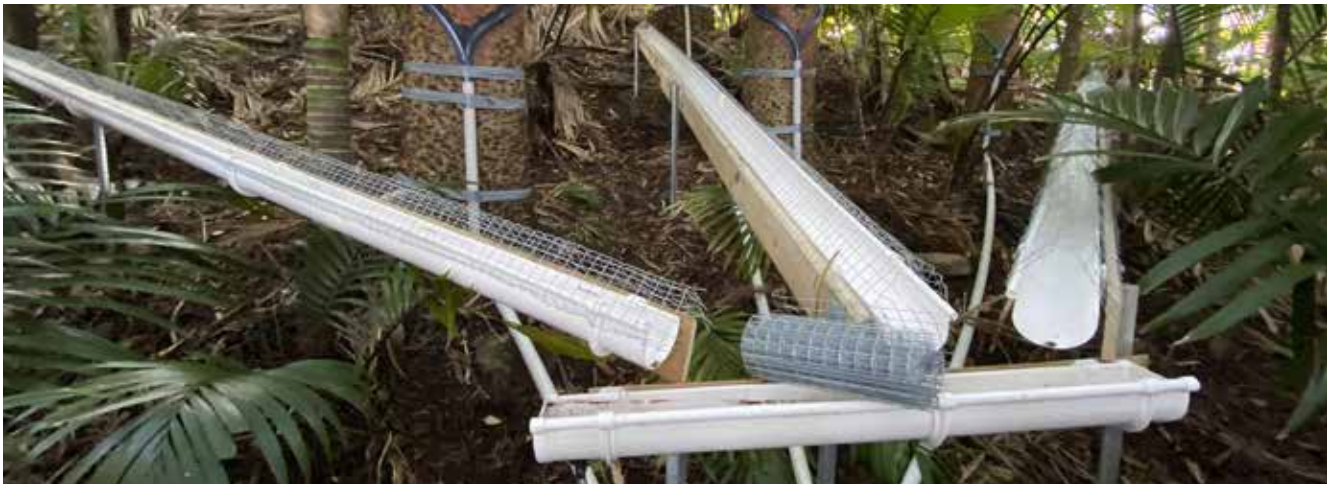
The layout of throughfall and stemflow measurement devices, set up in the forest canopy.
